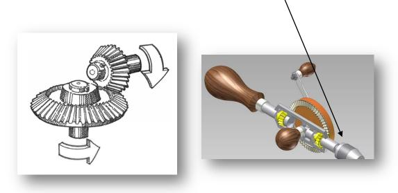
Bevel gears, like worm gears, use shafts at an angle of 90°. The hand drill shown uses them not only to change the rotary motion through 90°, but also, by using different sized gears, to increase the speed of rotation. The one shown gives a speed increase of 1:4.
